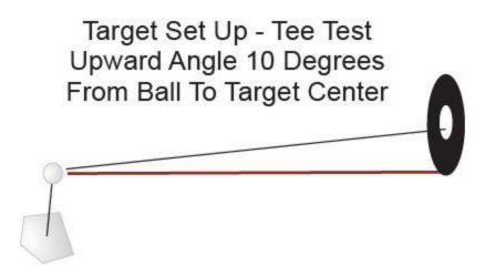
Set up the circle at a height so that the bottom of the target is the same height as the ball on the tee. This straight line is the 0 Line or 0 Degrees Launch Angle. The center will be approximately 10 Degrees and the top will be approximately 20 Degrees Launch Angle.
